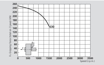
The data in the diagrams refer to 3-jaw-chucks, newly maintained according to their service manuals using SMW-AUTOBLOK K05 grease. The static and dynamic gripping forces have been measured using standard soft top jaws, placed in a position not exceeding the outer diameter of the chuck.
